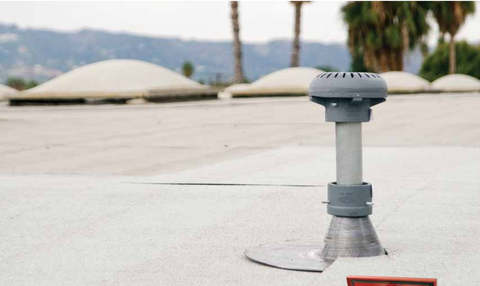
Stoneman® Roof Flashings are made of seamless lead and are available with counter flashing and vandal resistant flash hoods made of UV resistant PVC or cast iron.
